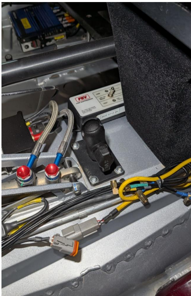
Figure 1. 25mm rubber ball securely attached to the tunnel
